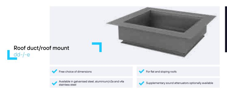
DL sound-absorbing roof mounts in a rectangular design are used to reduce the noise level of roof ventilators on the suction side. The housing, clad in mineral wool, is fitted with a sheet metal frame and four stays for the purpose of load bearing. It is securely mounted using a surrounding support flange. Optionally available with additional sound attenuators
