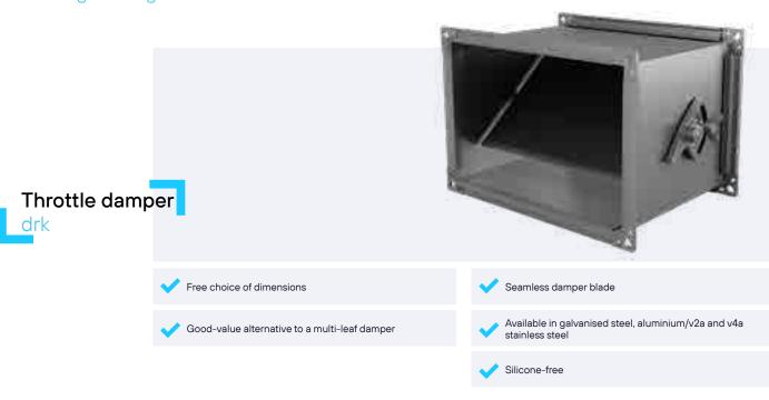
DL throttle dampers in a square design are used to regulate pressure and volumetric flow rate in ventilation systems. They are configured via a damper blade attached in the middle of the housing; in turn, this can be operated using a manual adjuster (including locking mechanism). Optionally, a motorised console can also be fitted to enable electric or pneumatic operation.
