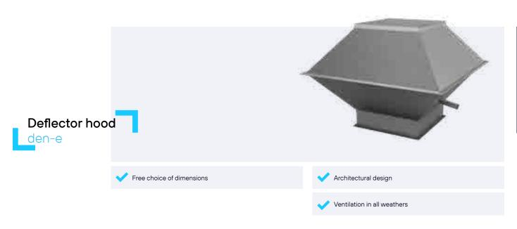
DL deflector hoods in a rectangular design are used on roofs to conduct away used air containing harmful substances. The characteristic shape of the deflector hood enables it to carry exhaust air upwards while simultaneously conducting precipitation outwards via an interior rain collection funnel.
